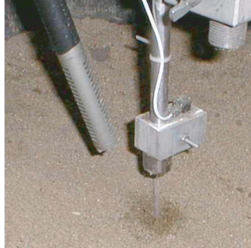
FIGURE 5: Data was taken in the laboratory using the setup shown. Sounds produced by the waterjet-soil-object interaction were recorded by the microphone on the left. The position and firing of the waterjet nozzle (right) were controlled by a computer.
