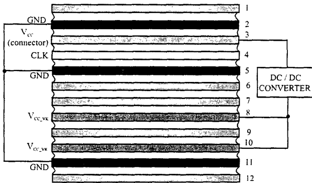
Figure 3. Layer stack-up for the CPU #2 PCB module.
