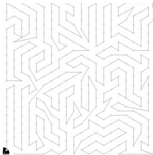
Fig. 9 - Optimized Path using a Physical Vehicle Heuristic.
