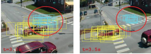
Fig. 3. An example of model selection. The circle shows particles with a wrong dynamics.
