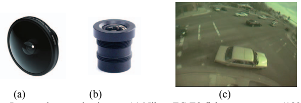
Fig. 1. Lens and a samples image. (a) Nikon FC-E8 fisheye converter (183° view-angle). (b) A \mu -video lens (150° view-angle). (c) A sample image captured with the \mu -video lens.
