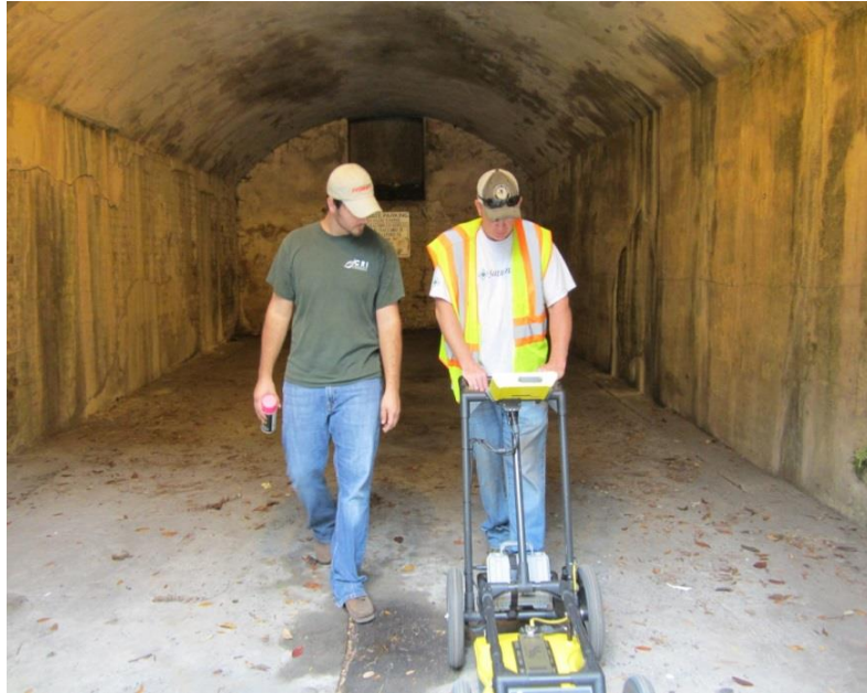
Figure 3.02 GPR Scanning of Vault 3
