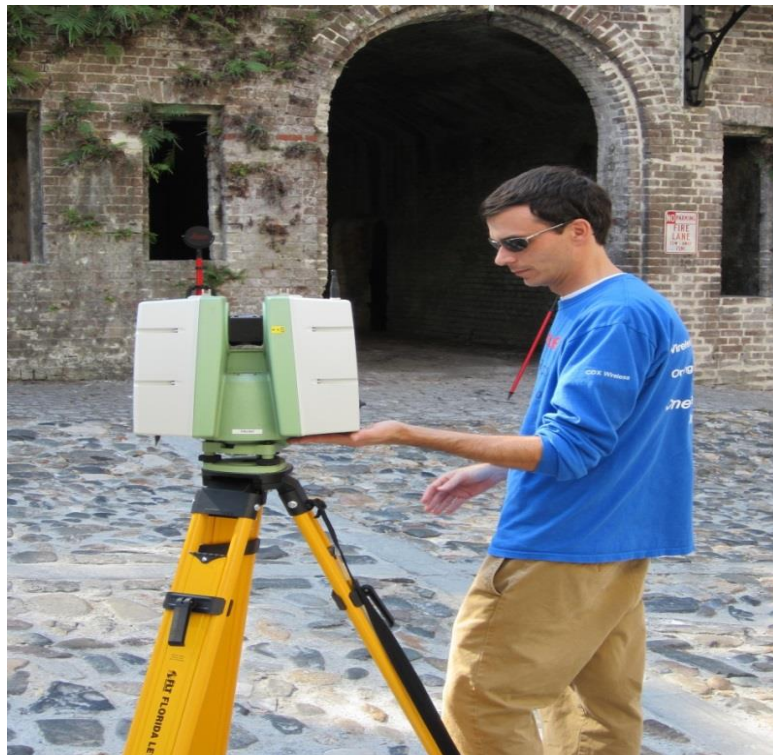
Figure 3.03 LiDAR Scanning of the Vaults
