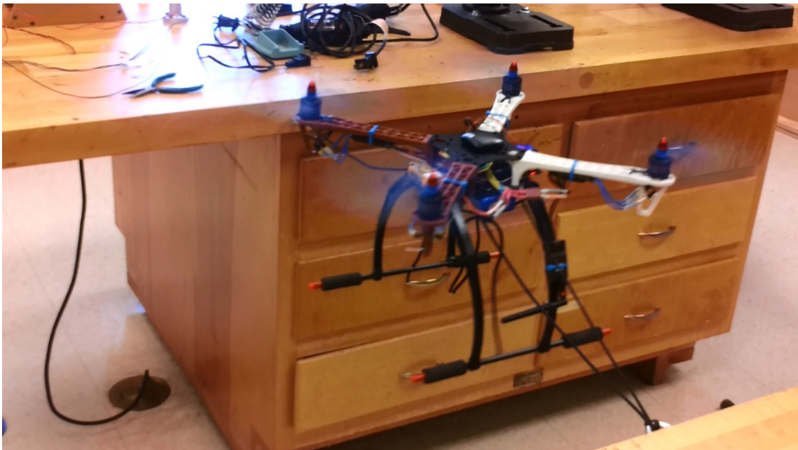
Figure 4.7. UAV flying in PID tuning harness
