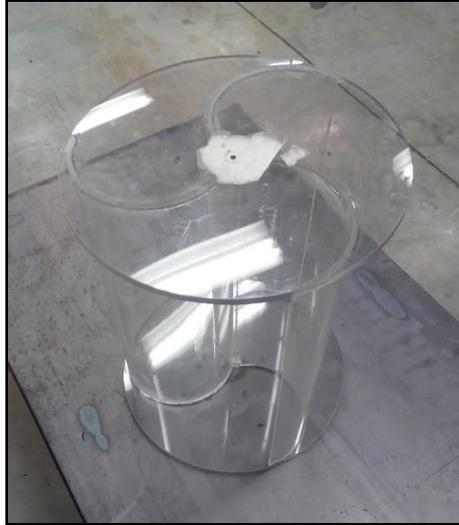
FIGURE 3-14: Fabricated Model of Semi Circular Bladed Rotor
