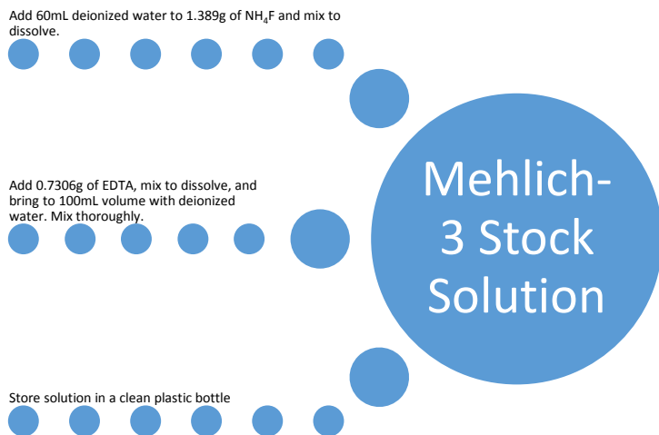
Figure 56: Steps to Create Mehlich-3 Stock Solution
