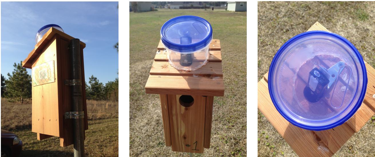
Figure 2. Three views of the modified nestbox.. Left: Back/side view showing the side window and the two U straps used to secure the box to the metal conduit pole. Middle: Forward view, showing the entrance and a camera mounted on the hinge inside the protective container. Right: View from above showing the camera rig through the protective plastic container
