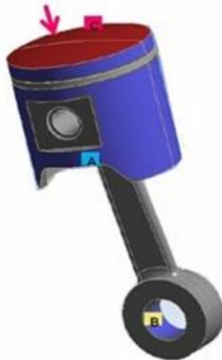
Figure 118 Static Structural Boundary Conditions
