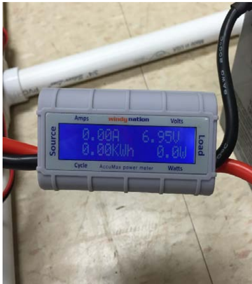
Fig. 5 Photo of in-line multimeter before the battery
