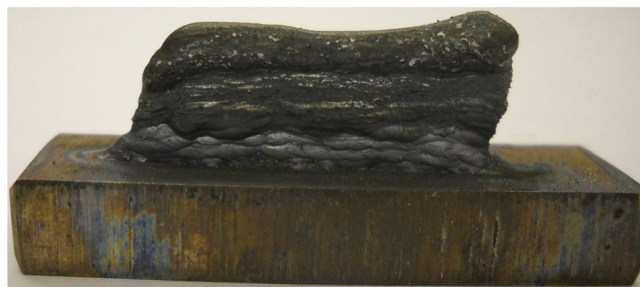
Figure 6. Thin wall multi-metallic sample.
