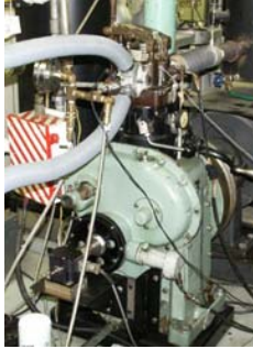
Fig. 2. Cooperative fuel research (CFR) engine.
