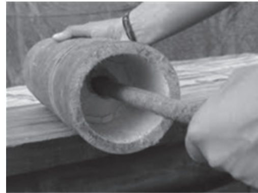
Figure 4. Drilling of culm diaphragm
