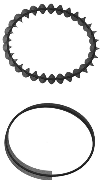
FIG. 8. Configuration of the rod equilibrium corresponding to the lower-energy circle in the bifurcation diagram of Figure 7. The rod centerline is indicated by a tube and the normal-vectors by a ribbon. The top figure shows the original normal vectors, which track the sugar-phosphate chains. The bottom figure shows the natural-frame normal vectors used in the computations (which are not periodic for this configuration).
