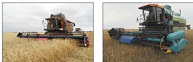
Fig. 1. Header with a stripper adapter: a) on the basis of Essil-760 with a header of 9-m width b) on the basis of Essil-740 with a header of 7-m width
