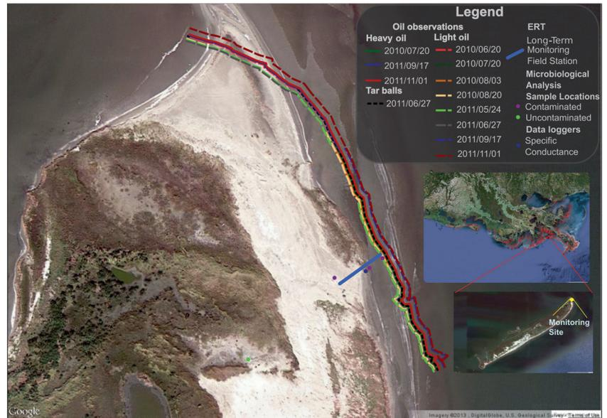
Figure 2. Map of the field site showing the locations of the microbiologic samples as well as the location of the resistivity line. Also included are the results of geochemical tests showing the presence of oil (Environmental Response Management Application, 2013).
