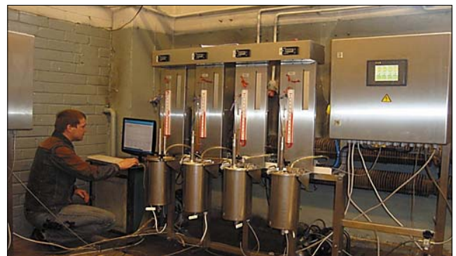
Fig. 2. A laboratory device consisting of four 5 l bioreactors
