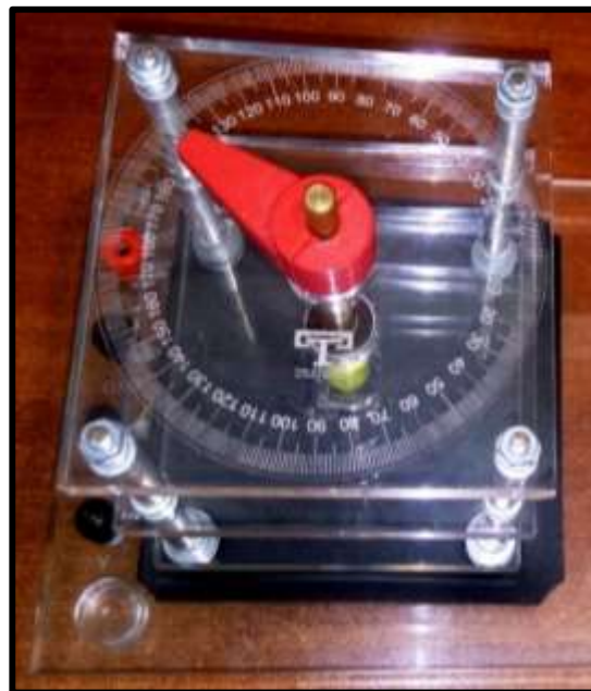
Figure 3. Absolute and angular position measurement prototype. Source: own.
