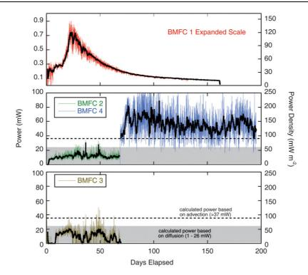
**Fig. 5** Power records from all BMFC deployments (raw data is shown with an overlay showing the 24 h running average in bold). Left axis shows actual power output and right axis shows power normalized to cross-sectional area. The upper panel has a magnified scale and shows the BMFC 1 results. Data from BMFCs 2–4 are shown in the lower panels. Shaded area is range of power predicted by diffusion calculations. Dashed line shows lower bound of power expected from advective flux (details in text).
