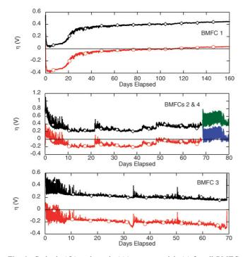
**Fig. 6** Cathode ( $\bigcirc$ ) and anode ( $\diamond$ ) overpotentials ( $\eta$ ) for all BMFC deployments based on open circuit potentials (*vs.* Ag/AgCl) observed during previous experiments at nearby seeps. BMFCs 2 and 4 are shown on the same plot (middle panel) since they are the same device that was recovered and then redeployed. The datalogger monitoring anode potential failed during the BMFC 4 deployment, so the record is incomplete.
