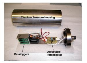
**Fig. 4** Photograph of potentiostat that controls the whole-cell potential and the titanium pressure housing.
