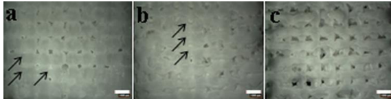
Fig. 6. Optical microscope images of the scaffolds after soaking in \alpha -MEM for (a) 1 day, (b) 5 days, and (c) 7 days (scale bar – 1mm). More pores are revealed with increased soaking time.
