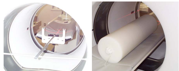
Figure 1: Setup for the NEMA 2001 sensitivity and count rate performance phantoms.
