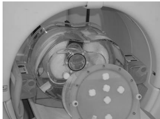
Fig. 1. Phantom setup, showing arms and out-of-field cylindrical phantom.
