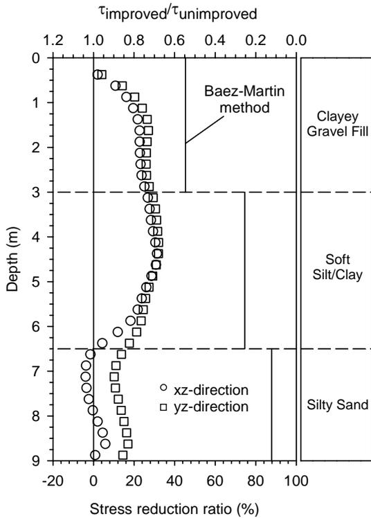
Figure 7. Shear stress reduction ratio; 3D analysis results compared with Baez-Martin design method
