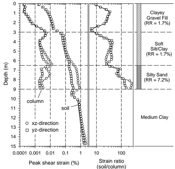
Figure 8. Comparison of the peak shear strains within the jet-grout column and the soil
