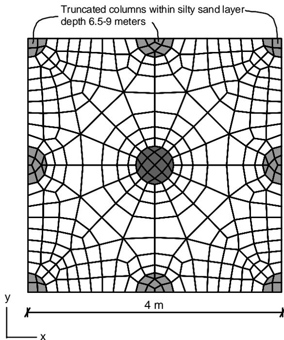
Figure 3. Plan view of the jet-grout column layout in the finite element model
