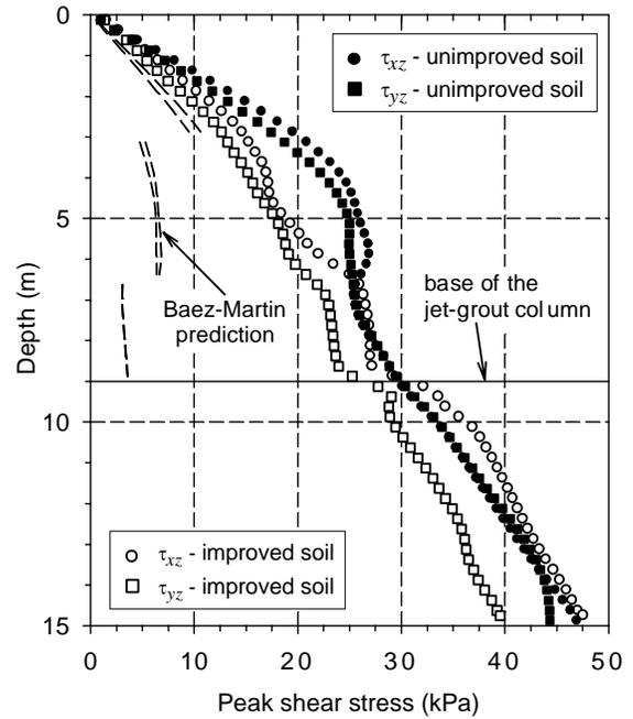
Figure 6. Calculated peak shear stresses in the improved and unimproved soil profiles
