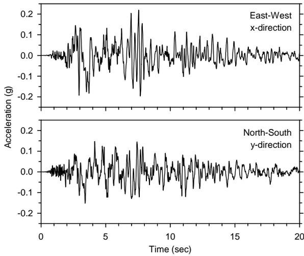
Figure 5. Components of base motion used in the analysis
