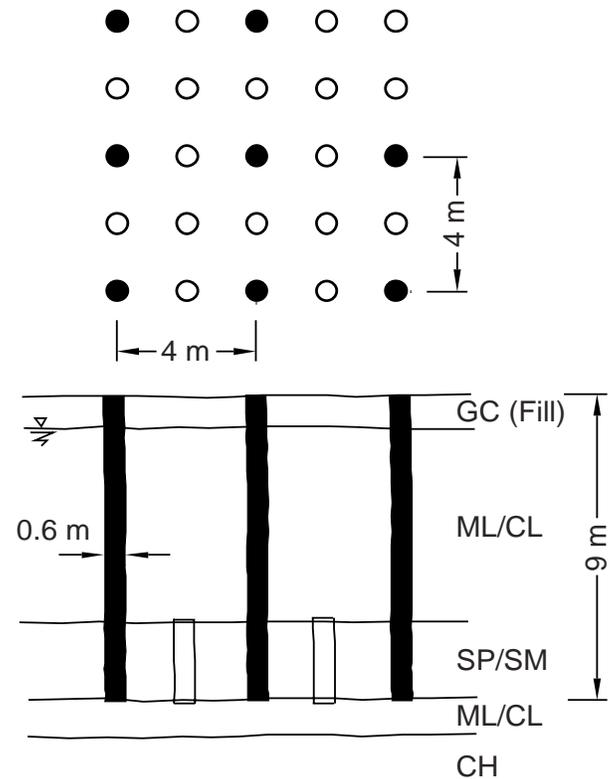
Figure 2. Jet-grout column layout
