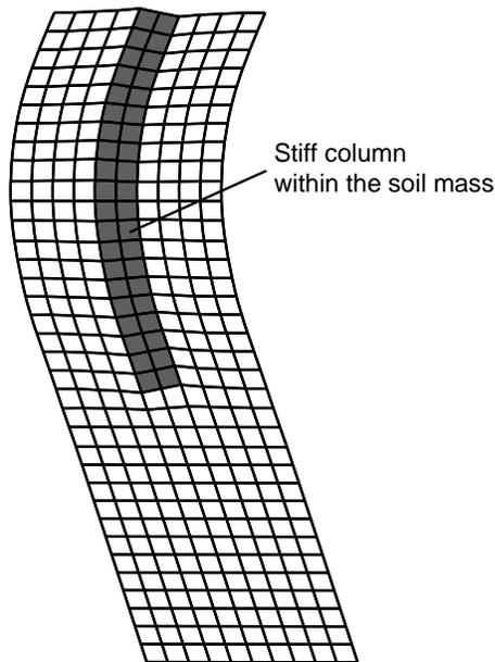
Figure 9. Stiff column deforming in flexure
