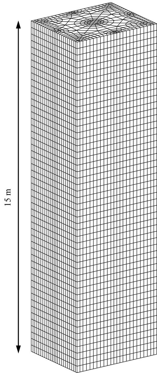
Figure 4. Finite element mesh of the 3-D model
