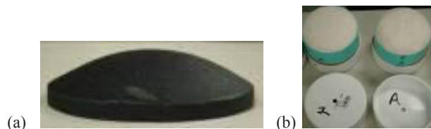
Fig. 1. Illustration of the EFP design (a) rubber coated flyer plate and (b) the hand packed EFP.
