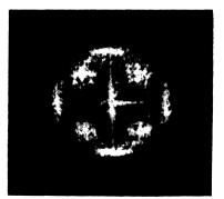
FIG. 2. Spatial power spectrum of the optical-intensity field corresponding to Fig. 1, shown on a logarithmic grey scale. The peaks at 45° are due to an imaging nonlinearity and are removed in the process of estimating the spectrum of h(x,y). The axial peaks correspond to the structure represented by Eq. (11), but are broadened.
