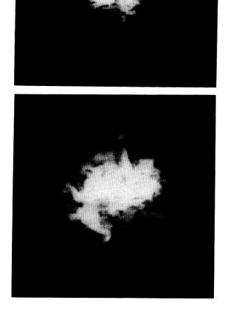
FIG. 6. Fluorescein-dye patch dispersal for  $\epsilon = 0.90$ . These optical-intensity distributions were obtained 2 and 4 s after the dye was introduced onto the surface.
