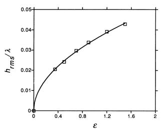
FIG. 5. Measured wave amplitude  $h_{\rm rms}$  (in units of the wavelength) as a function of the dimensionless driving amplitude. The variation is well approximated by a power law with exponent  $0.51\pm0.02$ .
