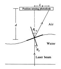
FIG. 4. Geometry of the method used to obtain the meansquare deformation  $\langle h^2 \rangle$ . The xz plane is shown.
