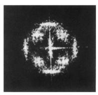
FIG. 2. Spatial power spectrum of the optical-intensity field corresponding to Fig. 1, shown on a logarithmic grey scale. The peaks at 45° are due to an imaging nonlinearity and are removed in the process of estimating the spectrum of h(x,y). The axial peaks correspond to the structure represented by Eq. (11), but are broadened.
