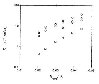
FIG. 7. Test of the fluctuating Stokes-drift model of capillary-wave transport: measured and calculated effectivediffusion coefficients  $(D_m, \text{ circles}; D_c, \text{ squares})$  as a function of the nondimensional wave amplitude.
