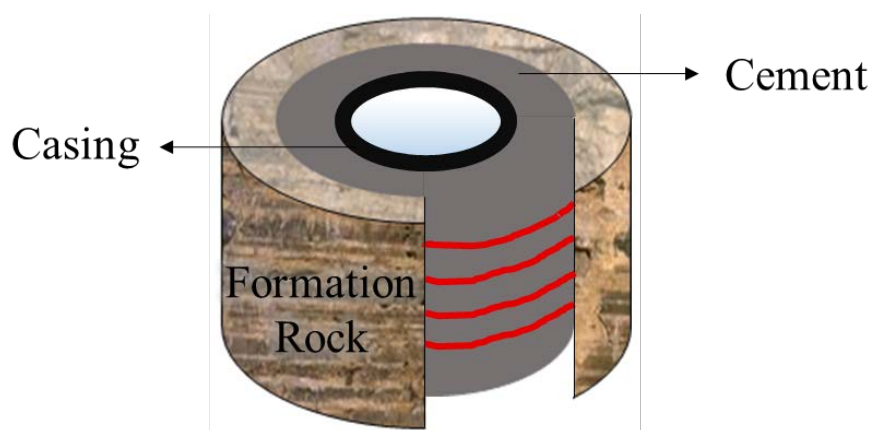
Figure 4. The dishing effect of axial cement shrinkage.
