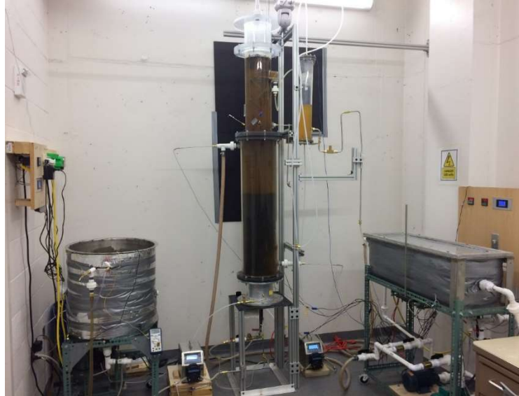
Figure 3. Two-Stages Expanded Granular Sludge Bed Reactor System
