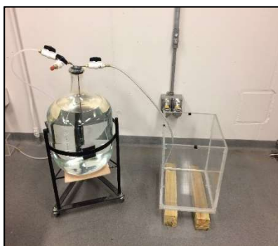
Figure 9. Water Displacement Method to Measure the Biogas Production Rate
