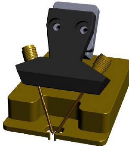
Figure 3.2. 3D model for D-probe with a mechanical base holder.
