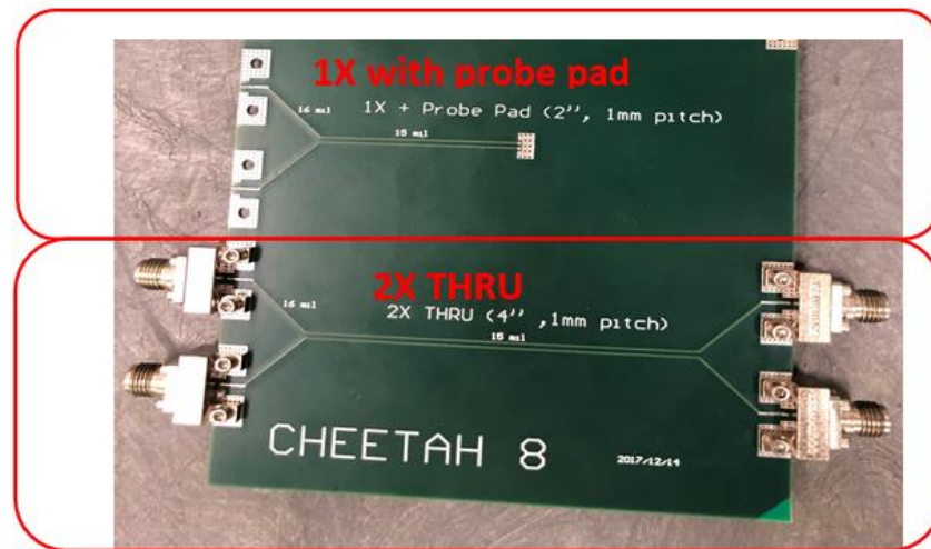
Figure 3.13. Top view of test board.
