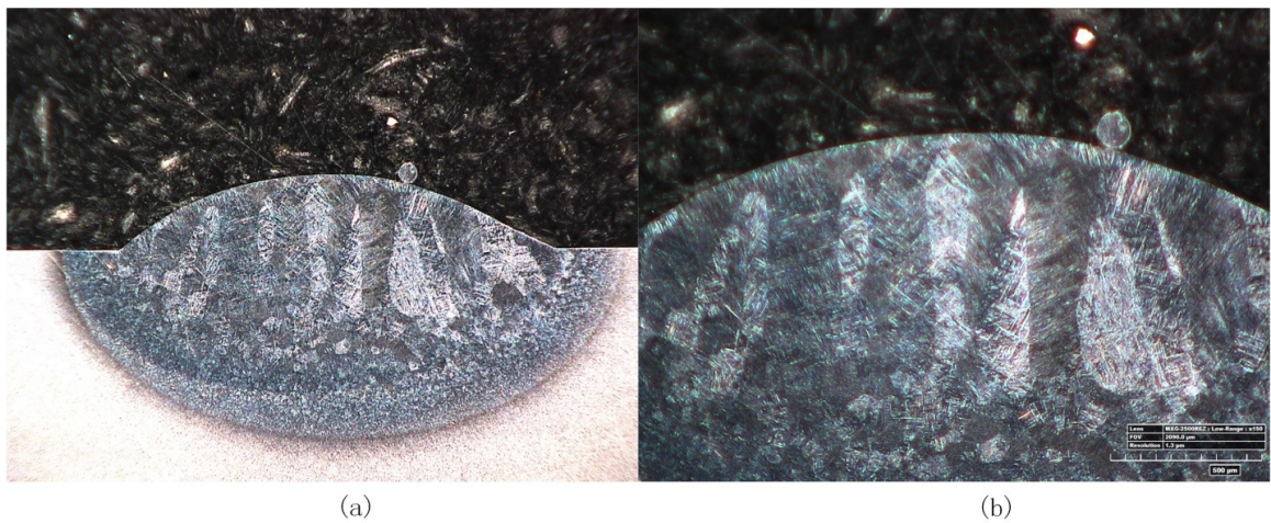
Figure 12. Ti-6Al-4V single-layer deposition grain morphology at (a) 50x and (b) 200x
