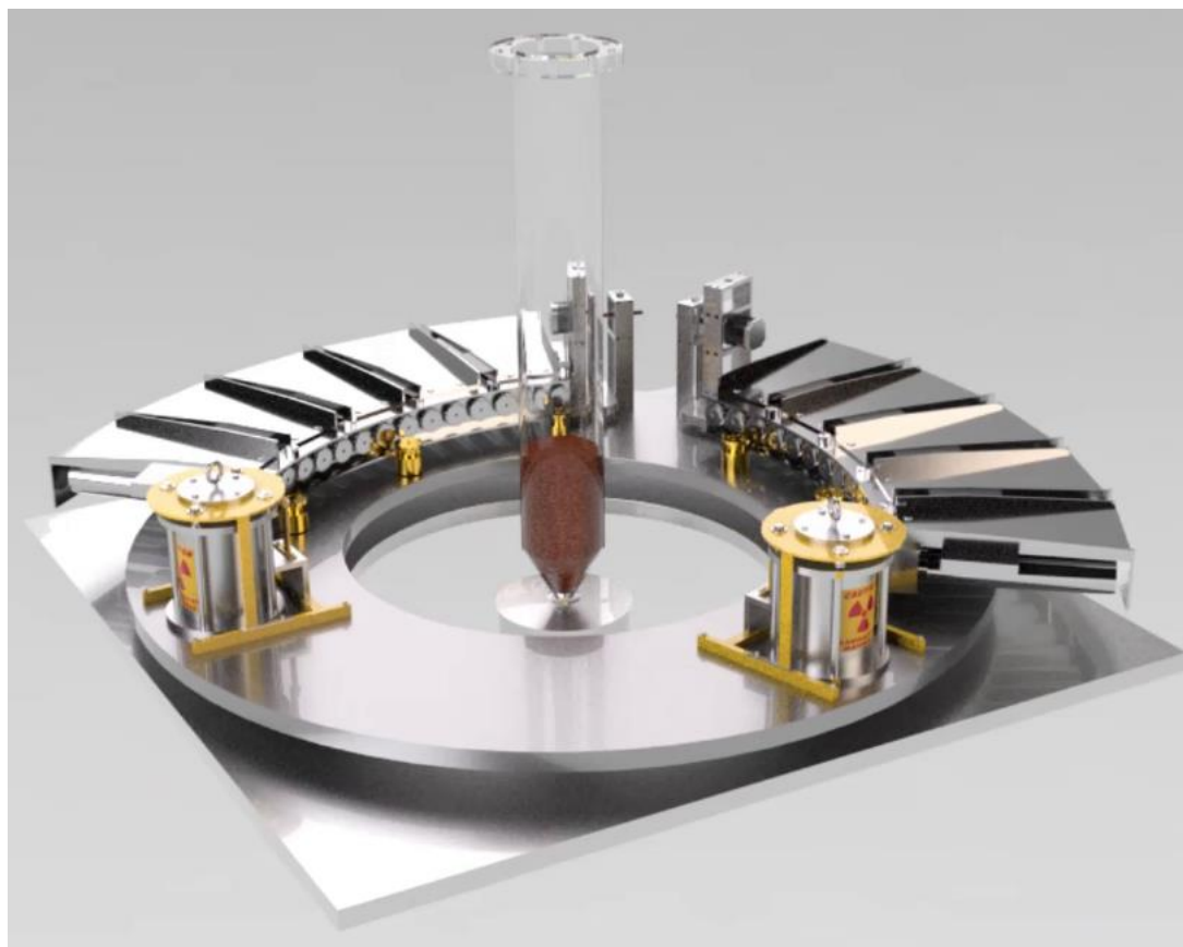
Figure 3.3. The platform of the DSCT technique and 6-inch gas-solid spouted bed inside the setup for the scan.
