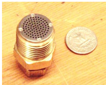
Figure 3.2. Gas distributor (stainless steel) used for 6-inch spouted bed to pass through the gas flow inside spouted bed.
