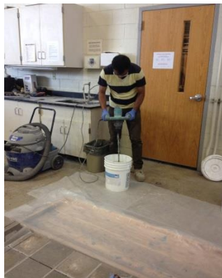
Mixing two part of epoxy
