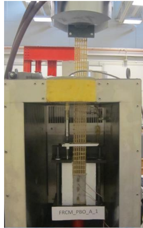
Heating and cooling chamber
