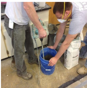
Preparing cementitious matrix
