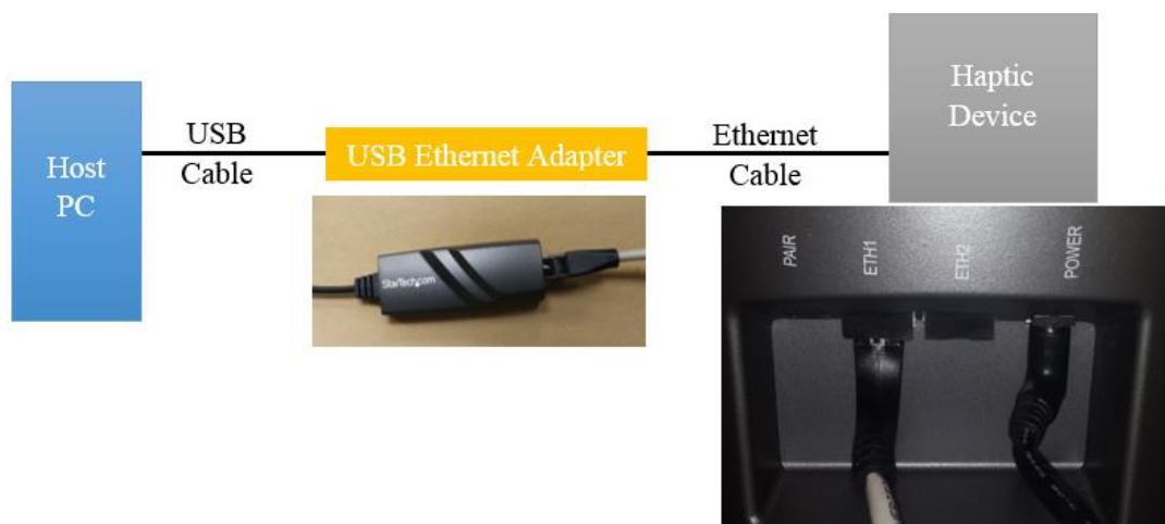
Figure 3.6 Haptic device to host PC connection
