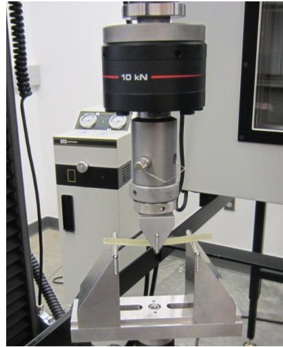
Figure 2.3. Experiment setup for three-point bending test
