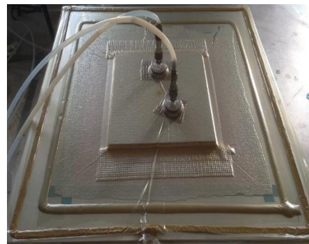
Figure 2.1. Schematic of out-of-autoclave process bagging assembly
