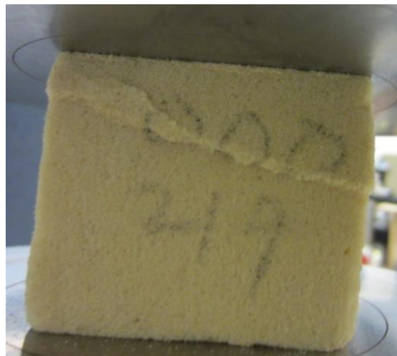
Figure 3.3. Representative failure mode of PU foam core specimens under compression
