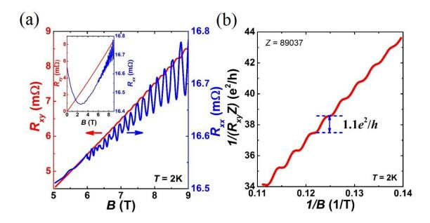
FIG. 7. (a) Longitudinal resistance  $R_{xx}$  and Hall resistance  $R_{yx}$  as a function of the applied magnetic field that perpendicular to the basal plane B//c at 2 K. Quantized plateaus in the  $R_{yx}$  are accompanied with the minima in  $R_{xx}$ . (b)  $1/ZR_{yx}$  as the function of inverse field. The step size  $\Delta(1/R_{xy})$  between the plateaus is approximately constant at  $1.1e^2/h$  per QL.
