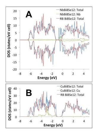
Fig. S5. DFT-GGA-calculated density of states (DOS) for (A) Nb-intercalated  $Bi_8Se_{12}$  and (B) Cu-intercalated  $Bi_8Se_{12}$ . The total and the partial (Nb or Cu) density of states are plotted with a blue and green line, respectively. For comparison, the density of states of undoped  $Bi_8Se_{12}$  where the FL is moved up into the conduction band via a rigid-band (RB) shift is plotted with a red line. The FL is at 0 eV in all plots.
