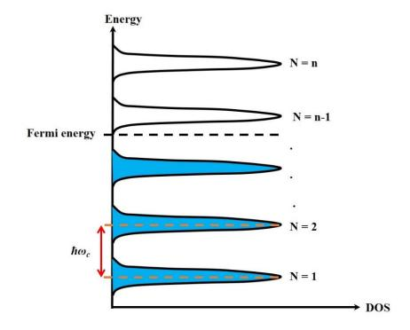
Fig. 2.2. Formation of Landau levels under the influence of external magnetic field as a function of DOS. Landau levels are separated by  $\hbar\omega_c$ . Since  $\omega_c$  is directly proportional to *B*, the energy gap in-between Landau levels increases as *B* increases. Landau levels below the Fermi level are filled with electrons.
