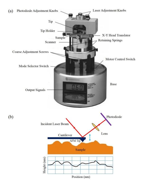
Fig. 4.7. AFM measurement. (a) The instrument is set into the tapping mode and the tip, laser, mirror, and photodiode must be aligned before the measurement. (b) The laser beam is focused on the back of a cantilever that moves vertically on the surface of a sample and the deflections of the beam are detected by a position-sensitive photodiode to track the surface for imaging and measuring. Fig. (a) is adopted from the Digital Instruments Multimode<sup>TM</sup> SPM Instruction manual.
