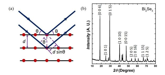
Fig. 4.2. XRD measurement. (a) Graphical representation of Bragg's law. (b). Typical powder-XRD diffractogram of  $Bi_2Se_3$  TI. Selected peaks are indexed with the Miller indices.
