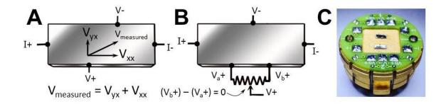
Fig. S4. Hall resistivity measurement. (A) Contact leads for four-wire Hall measurement on a sample bar. Offset  $V_{xx}$  is due to a longitudinal resistivity. (B) Offset nulling can be performed with five-wire Hall measurement. The Hall voltage  $V_{yx}$  can be obtained by measuring the voltage dropped between V- and V+. (C) The setup of the five-wire Hall measurement. The Hall measurements for two samples can be performed simultaneously.
