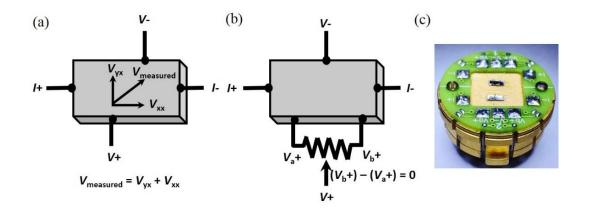
Fig. 4.6. Hall resistivity measurement. (a) Leads attached on bar sample for four-probe Hall resistivity measurements. (b) Offset nulling is performed with a five-probe Hall resistivity measurement. The potential difference between V+ and V- is Hall voltage  $V_{yx}$ . (c) Five-probe Hall resistivity measurement with samples mounted on ACT sample puck.
