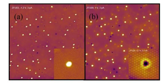
FIG. 2. STM topographic images on  $160 \times 160 \ \mu\text{m}^2$  area showing the (a) filled stated at a bias voltage of -1.2 V and (b) unfilled stated at a bias voltage of +1.0 V. The inset of (a) and (b) show the bias-independence of bright protrusions and the Mn-substituted on Bi site, respectively.
