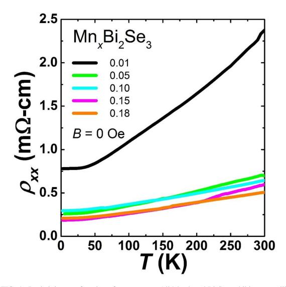
FIG. 4. Resistivity as a function of temperature. All Mn-doped Bi<sub>2</sub>Se<sub>3</sub> exhibits a metallic behavior.
