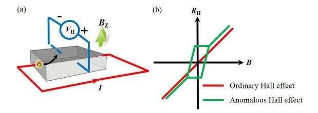
Fig. 2.3. Hall measurement. (a) Hall effect measurement setup. (b) Magnetic field dependence of Hall resistance,  $R_{\rm H}$  in ordinary Hall effect (red line) and anomalous Hall effect (green line).
