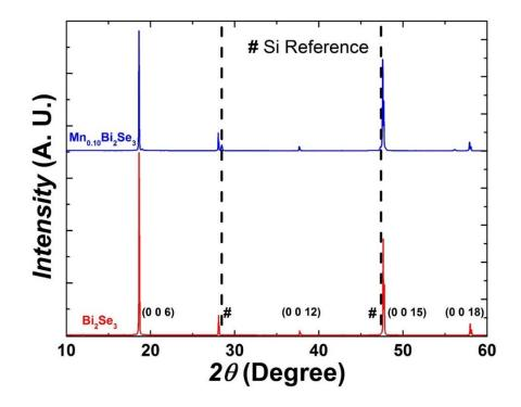
FIG. 1. Comparison of the reflected XRD peaks between the host compound  $Bi_2Se_3$  and Mn-doped  $Bi_2Se_3$  with Si peaks serve as the reference. The XRD peaks of Mn-doped  $Bi_2Se_3$  are shifted to the left, suggesting the increased of the *c*-lattice parameter.
