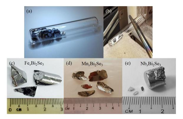
Fig. 3.2. Resultant ingots of chemically doped TIs. (a) A stoichiometric mixture of  $Bi_2Se_3$  inside a sealed evacuated quartz tube. The resultant ingots of (b)  $Bi_2Se_3$ , (c) Fe-doped  $Bi_2Se_3$ , (d) Mn-doped  $Bi_2Se_3$  and (e) Nb-doped  $Bi_2Se_3$ , respectively.
