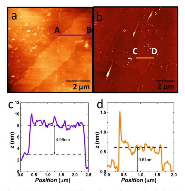
Figure 3. AFM micrographs of (a)  $Bi_2Se_3$  nanoribbon exfoliated onto glass with 100 V of applied voltage. (b) graphene that exfoliated onto the Si substrate. (c) From the AB-line scan of the post-processing micrograph, the thickness of the  $Bi_2Se_3$  nanoribbon is found to be  $4.99 \pm 0.50$  nm. (d) The thickness of the graphene flake indicates in panel (b) is 0.61 nm.
