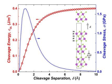
Figure 2. Calculated cleavage energy (circles, solid line) and cleavage stress (dotted line) as a function of cleavage separation in (0001)  $Bi_2Se_3$ . The inset illustrates the size view of the Se-Bi-Se-Bi-Se quintuple layer  $Bi_2Se_3$  model structure. Each quintuple layers are separated by 2.5 Å van der Waals gaps.
