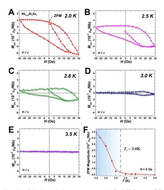
Fig. S3. Zero-field Magnetization measurement. (A)-(E) MH loop at different temperatures. The hysteresis loop is only observed for temperatures below  $T_c$ . (F) ZFM magnitude as the function of temperatures. Nonzero magnetization is observed for temperature below  $T_c$ .
