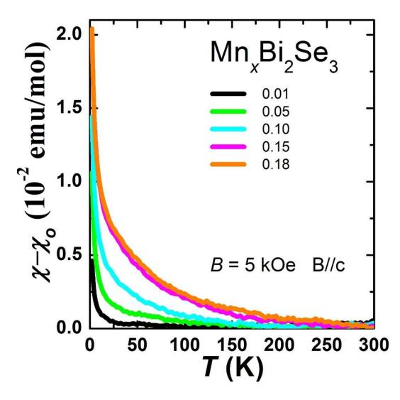
FIG. 3. Temperature-dependent magnetic susceptibility  $\chi$  measured at 5 kOe for the crystal aligned with the magnetic field perpendicular to the basal plane B//c. The ground state of the Mn-doped crystals is paramagnetic.
