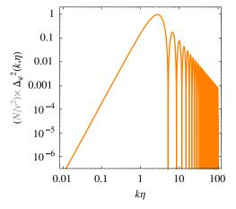
FIG. 2 (color online). The dimensionless power spectrum of the scalar-field fluctuations at a given scale and time:  $(N/v^2)\Delta_{\varphi}^2(k,\eta) \equiv (N/v^2)k^3P_{\varphi}(k,\eta)/(2\pi^2)$  in a radiation-dominated universe. This spectrum depends only on  $k\eta$ , and is thus self-similar. There exists an additional cutoff (not apparent in this plot) at  $k\eta = \eta/\eta_t \gg 10^2$ , set by the initial time of the phase transition  $\eta_t$ .
