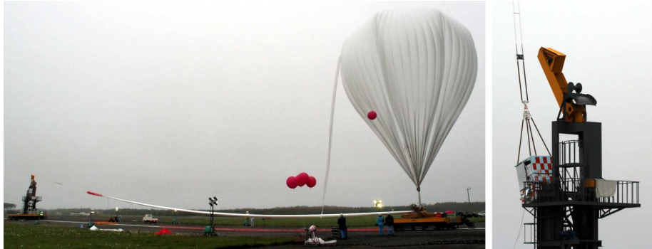
Figure 4: Left: pGAPS on the launcher and inflated balloon right before launch. Right: pGAPS during take off.
