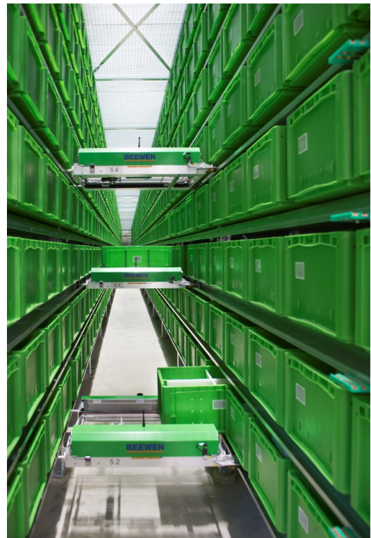
Fig. 3. Closer view of an aisle with shuttles (Source: Vanderlande industries)
