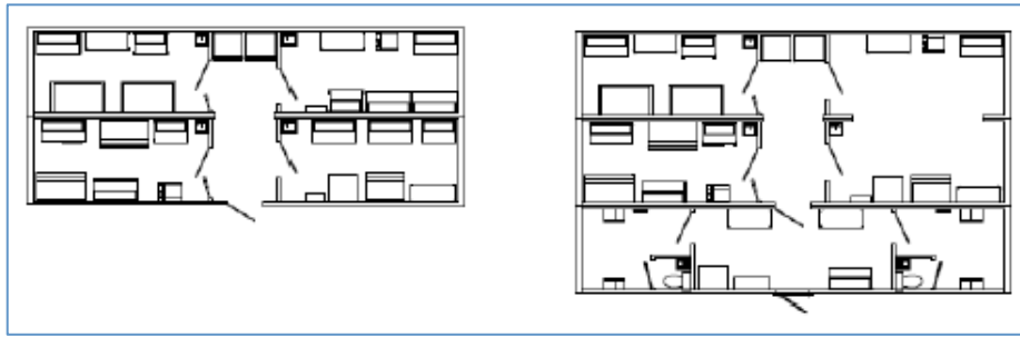
Figure 1. Modular P&G approach where a facility grows from two to three modules (Source: [9])
