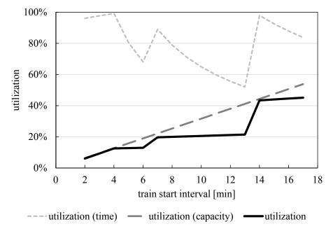
Figure 3: Impact of tugger train start interval on utilization (overall as well as of driver's working time and tugger train's transport capacity)
