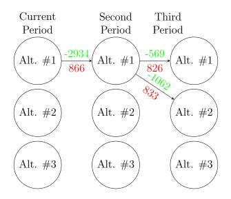
Figure 2: Alternative solutions for the example, depending on the relayout cost. Green values show the change in total cost of loaded and empty travel, whereas red values show the change in the cost due to waiting
