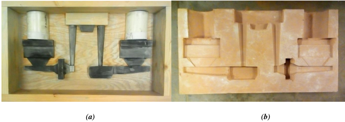
Figure 5. (a) 3D-printed patterns in a wooden flask and (b) corresponding half of a vertically parted no-bake sand mold.
