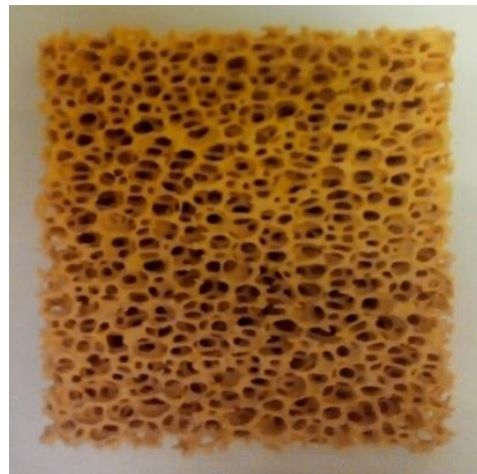
Figure 2. Zirconia foam filter: 10 ppi (10 cm X 10 cm X 2.5 cm).
