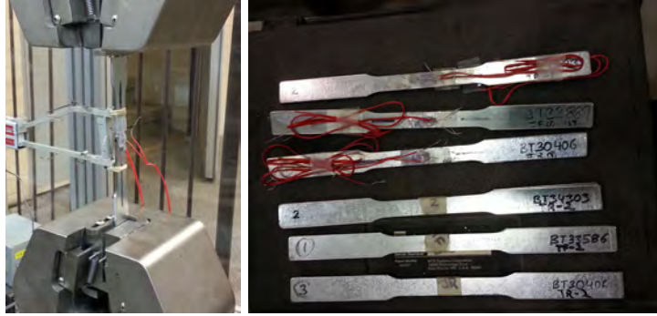
Figure 12: Tensile coupon testing process
