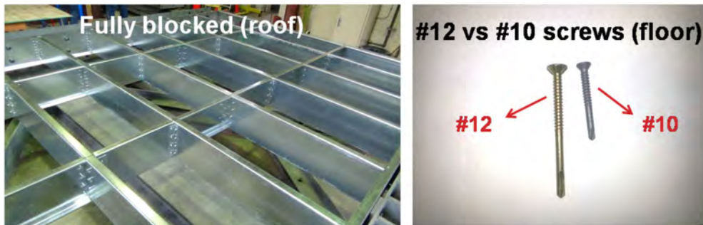
Figure 10: Diaphragm modifications for Part 2 of experimental program
