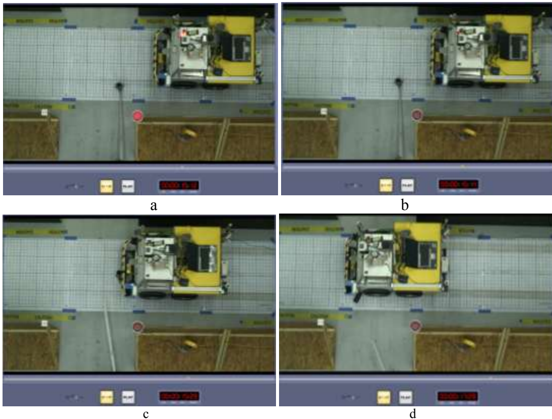
Figure 5 – Snapshots from the overhead video showing when: (a) the test piece crosses the photo-sensor, (b) the test piece is detected by the AGV safety sensor, (c) the AGV hits the test piece (or when the test piece stops in the AGV path), (d) the AGV stops.
