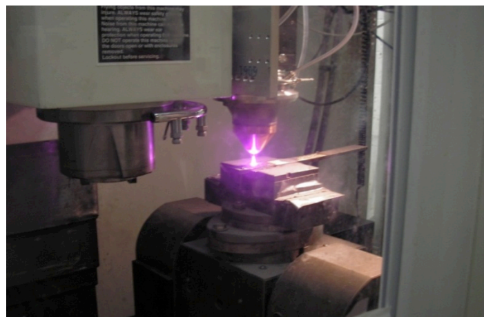
Fig. 1: Laser Aided Manufacturing Process deposition system
