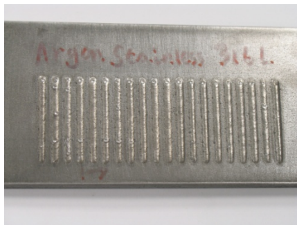
a. Argon shield gas sample
