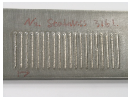
b. Nitrogen shield gas sample
