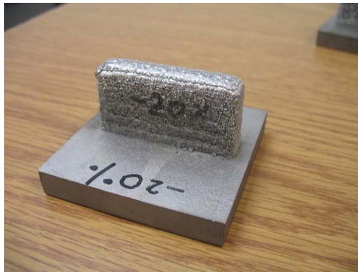
(b) Sample produced at -20% laser power
