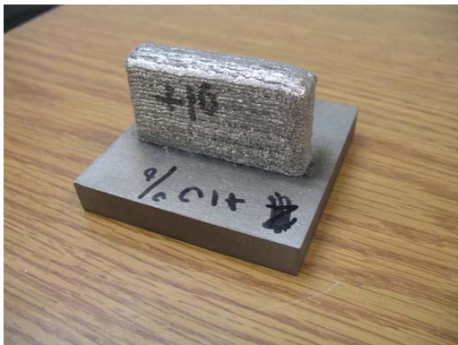
(e) Sample produced at +10% laser power
