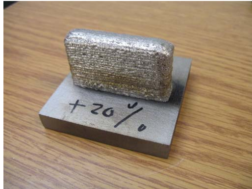
(f) Sample produced at +20% laser power
