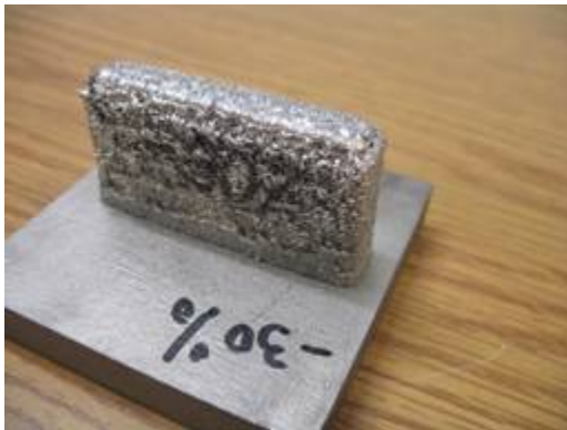
(a) Sample produced at -30% laser power
