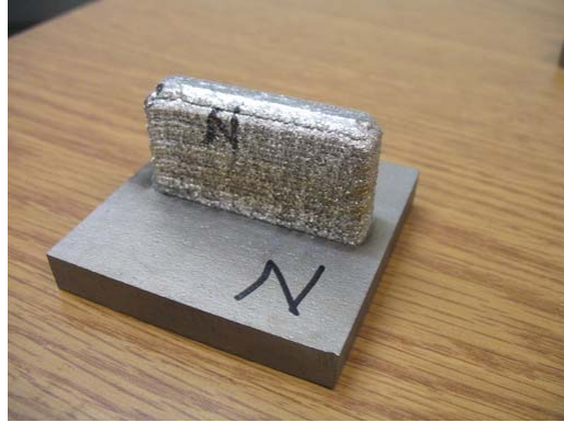
(d) Sample produced at nominal laser power
