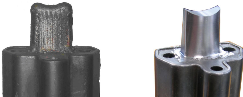
Figure 1. The die after repair by laser deposition and machined by CNC
