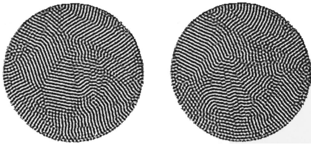
FIG. 2. Spatiotemporal chaos in rotating Rayleigh-Bénard convection shown at two different times. Patches of rolls at different angles invade each other as time proceeds. Courtesy of G. Ahlers.
