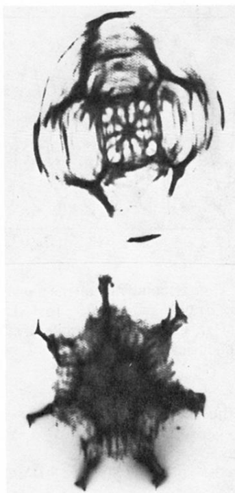
FIG. 1. Digitized optical intensity patterns for the (4,3) and (7,2) modes, respectively. The first index gives the number of angular maxima.
