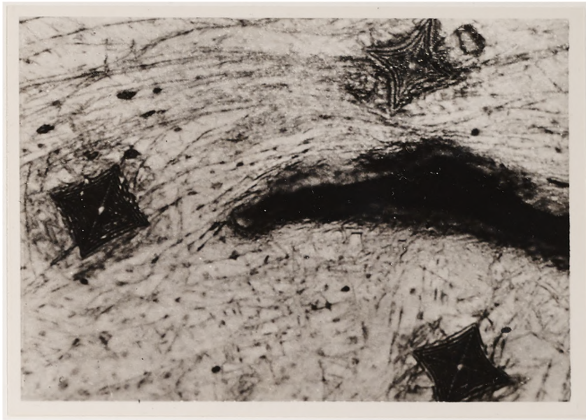
Figure 12. Microhardness Impressions Around the End of a Crack in the 40 Percent Cold Rolled Annealed Sponge. 650X.
