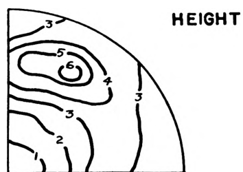
FIGURE 36. THE (10\bar{1}0) POLE FIGURE FOR 40 PERCENT COLD-ROLLED SPONGE OBTAINED BY MEASUREMENT OF PEAK AREA AND PEAK HEIGHT.
