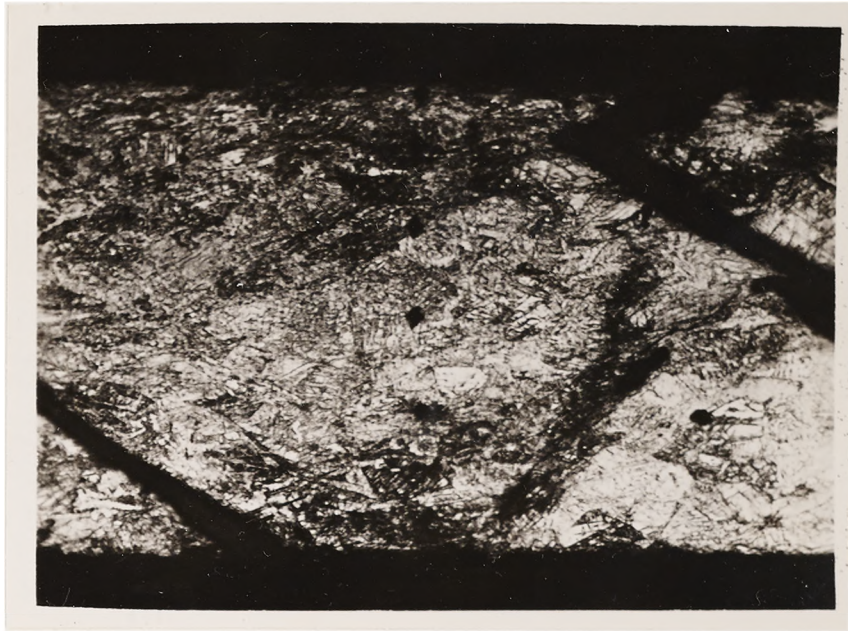
Figure 10. Microhardness Impressions in 40 Percent Cold Rolled Annealed Cobalt Sponge. 100X.
