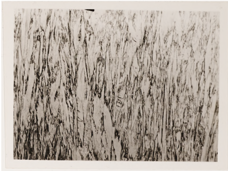
Figure 2. Microstructure of Electro-deposited Cobalt Parallel to Direction of Crystal Growth. 100X.
