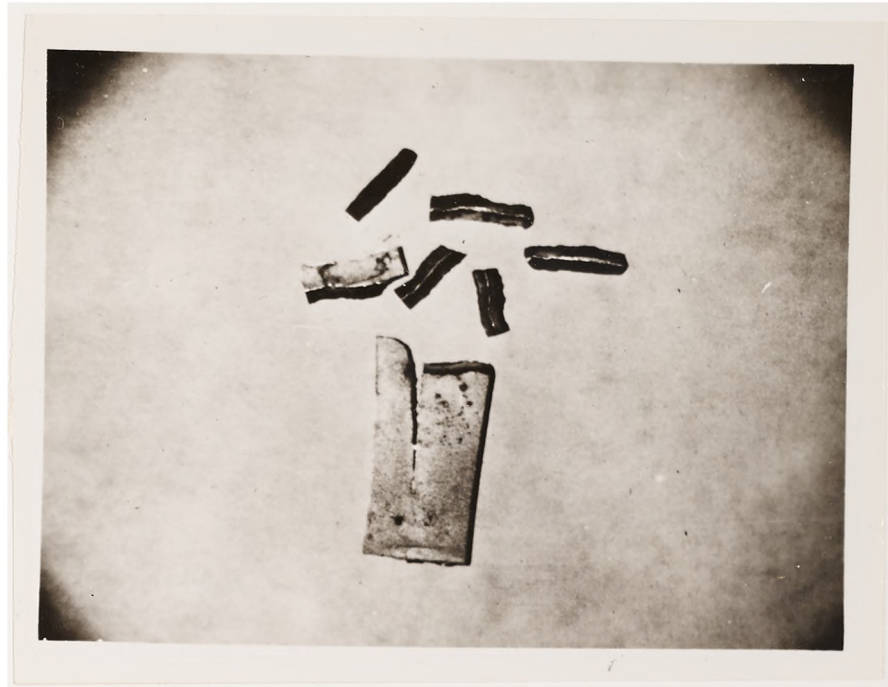
Figure 1. Electrodeposited Cobalt Reduced 11 Percent by Cold Rolling. 2X.
